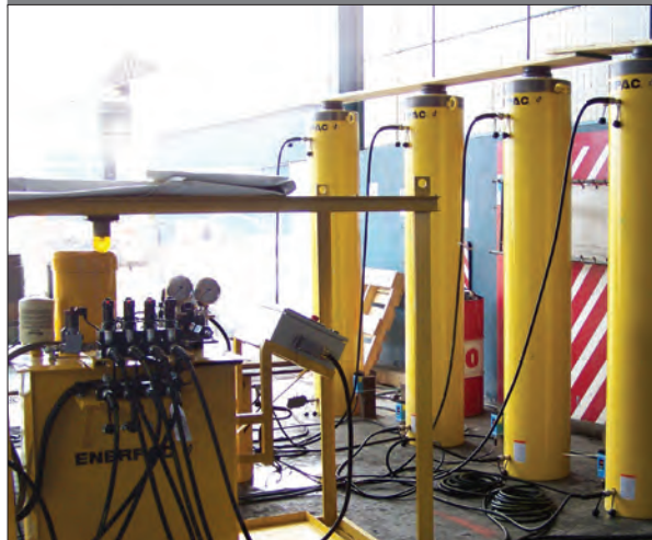
▲ Custom 500-ton cylinders with 72-inches of stroke for lifting electric rope shovels.
