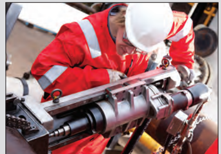
▲ High torque portable drilling machines.
