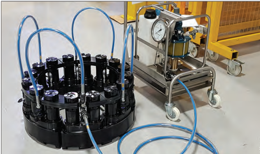
▲ Multi Stud Tensioning Set-Up.
