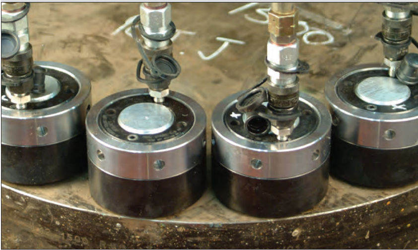
▲ Tensioning with hydraulic nuts.
